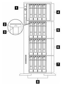
Figure 3. Front view of server models with sixteen 3.5-inch drive bays
