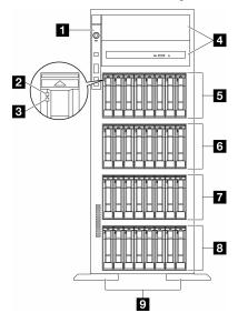
Figure 4. Front view of server models with thirty-two 2.5-inch drive bays
