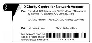
Figure 19. Lenovo XClarity Controller network access label on the pull-out information tab
