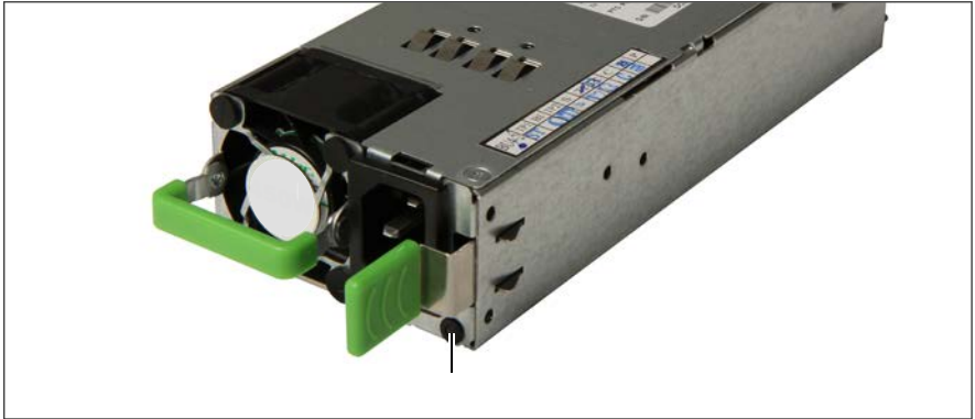
Figure 20: PSU status indicator (AC PSU)
