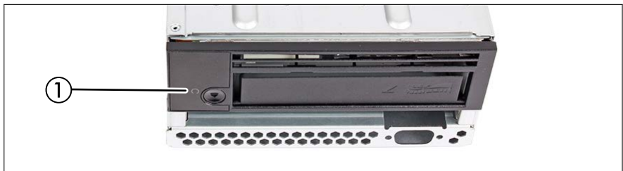
Figure 14: Indicators on the LTO drive
