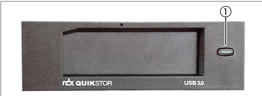
Figure 13: Indicators on the RDX drive
