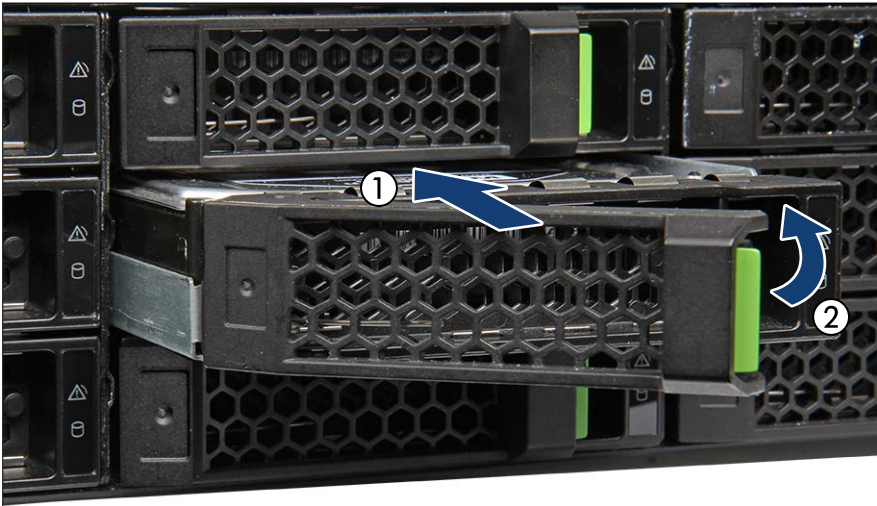
Figure 38: Installing the 3.5-inch HDD module
