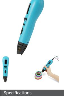
Case material: plastic Model build size: free form Filament: ABS, PLA, 1.75mm Nozzle diameter: 0.90 mm ceramic Screen: 0.91" OLED Screen Extruder temperature: 170 230 (adjustable) Moulding speed: adjustable Power consumption: 12 VDC up to 2A, adapter for 100-250 V AC
