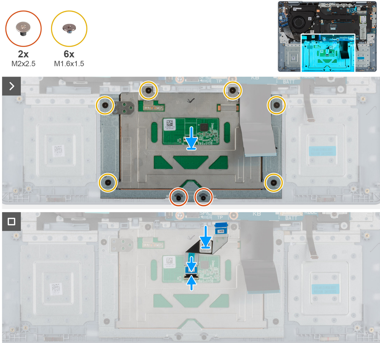
Figure 39. Installing the touchpad
