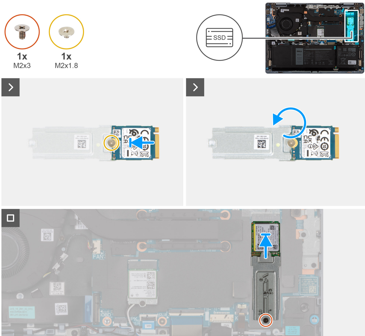
Figure 23. Installing the solid-state drive
