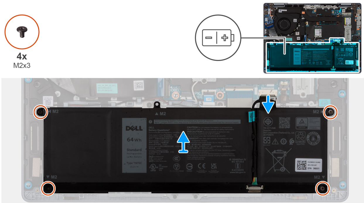
Figure 18. Removing the battery
