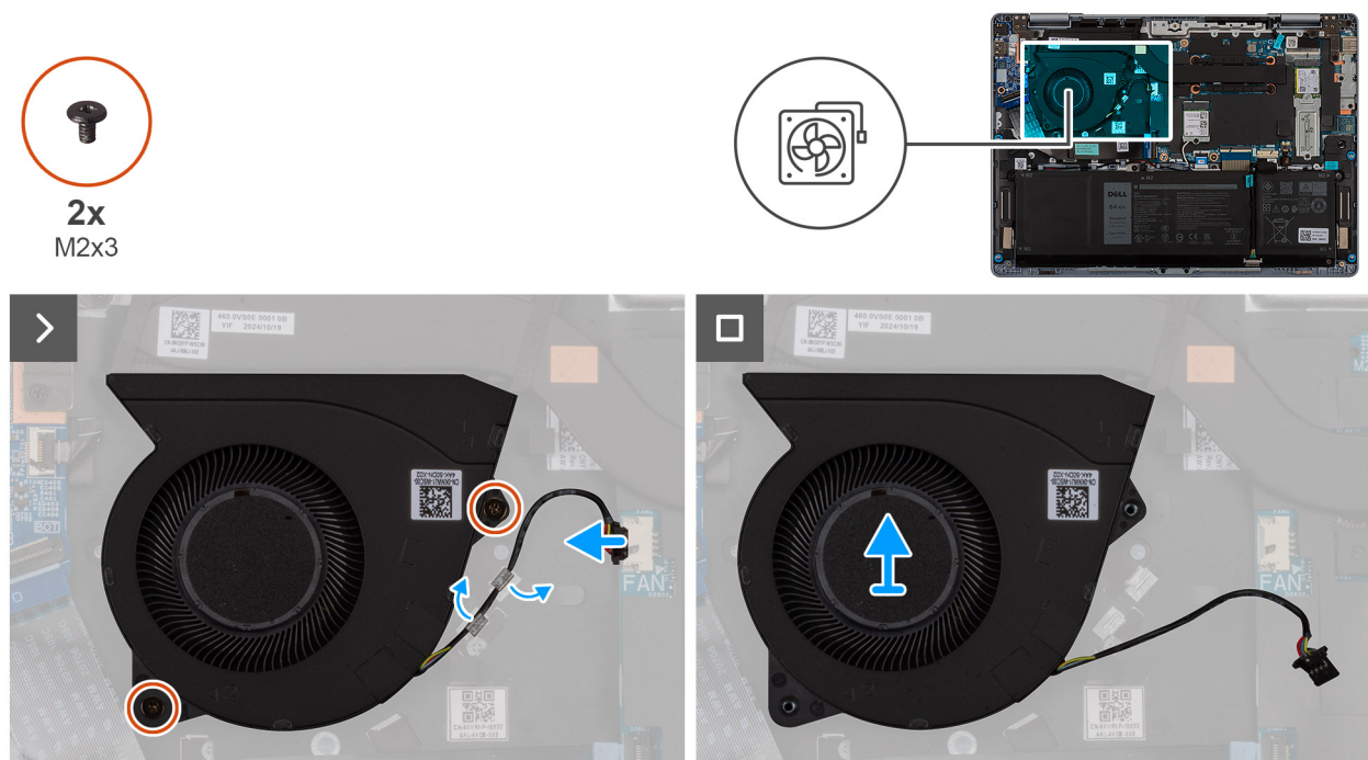
Figure 26. Removing the system fan
